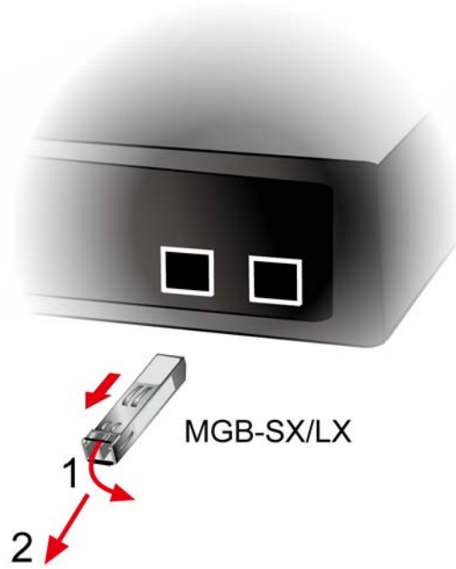
Figure 2-1-8 How to Pull Out the SFP Transceiver
