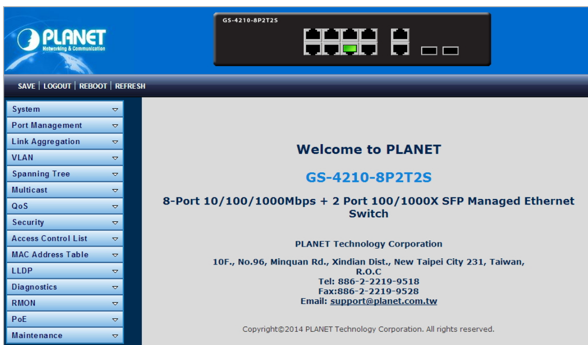
Figure 3-1-4 Web Main Screen of Managed Switch
